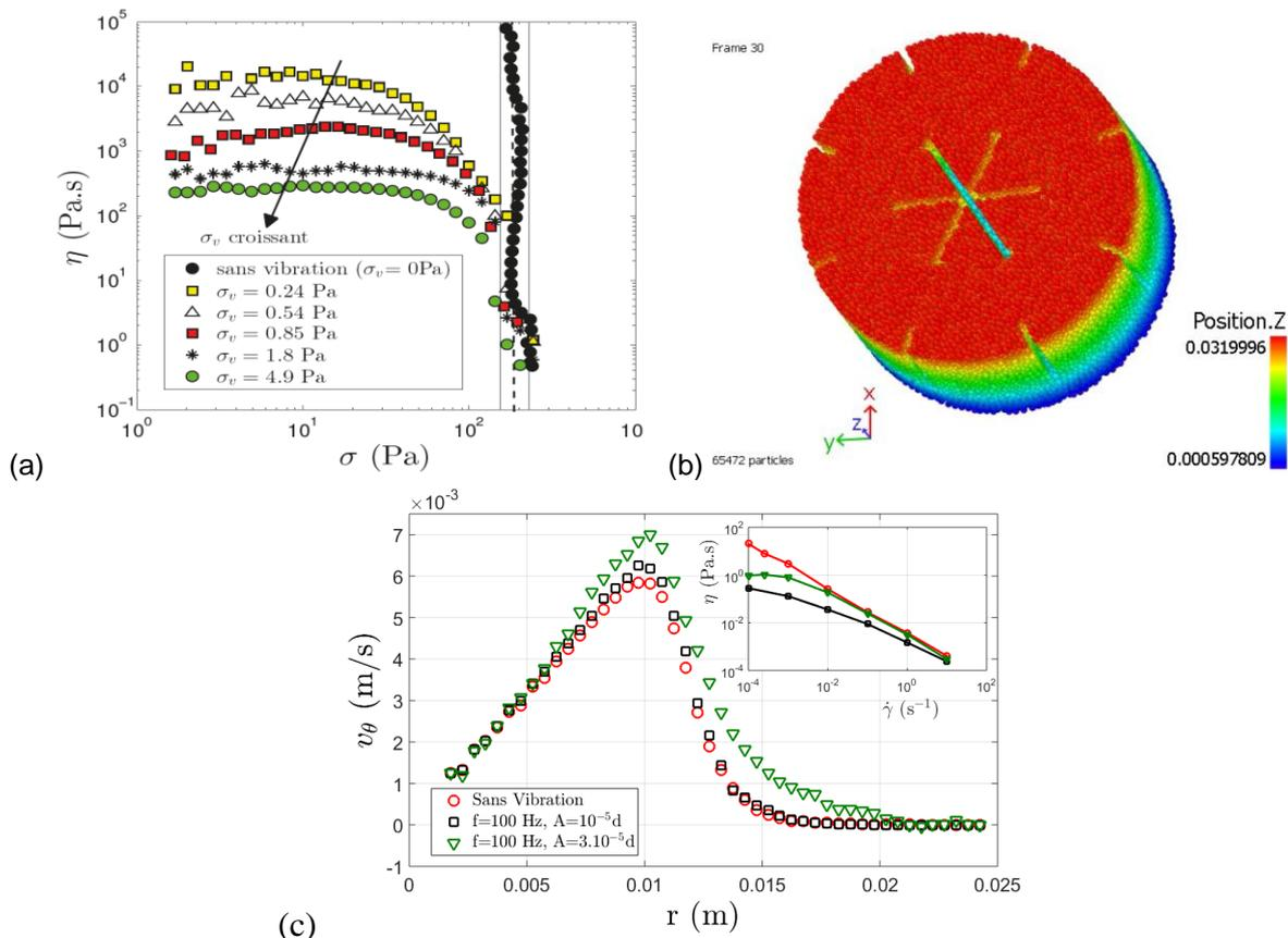
Figures: (a) Flow curves of granular dispersions, with and without vibrations, obtained with classical rheometry, (b) “Numerical rheometer” (DEM simulation) and (c) Example of velocity profiles obtained in DEM for various vibration energies.
